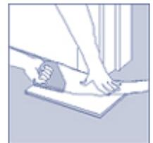
Check the wall where you are starting the installation and make sure it is squared to the opposite wall. Simply measure the room from the opposite ends of the wall to the firewall. If measurements are different make the necessary adjustments on the first row. Make sure that the widths of the first and last rows planks are identical or greater than 1/3 of the plank.
